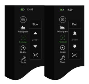
Tap the Focuser icon in the left Auxiliary Tools area to show the Focus Control Pad, switch the move step size which is set in the Fine (Slow) Step and Coarse (Fast) Step options by tapping the text button 'Slow'/'Fast'.
