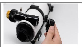
Remove the coarse adjustment knob of the telescope focuser with a suitable sized wrench.
