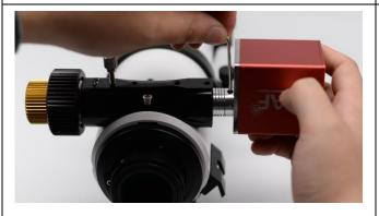
Attach the bracket to the focuser and then fix it to the EAF body with the screws.
