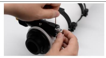
Install the flexible coupling on the telescope focuser shaft and tighten the lock screw.
