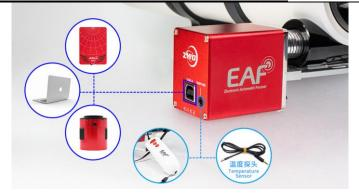
Connect the EAF to the ASIAIR/computer/cooled camera, hand controller or the temperature sensor.
