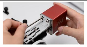
Attach the bracket to the focuser and then fix it to the EAF body with the screws.
