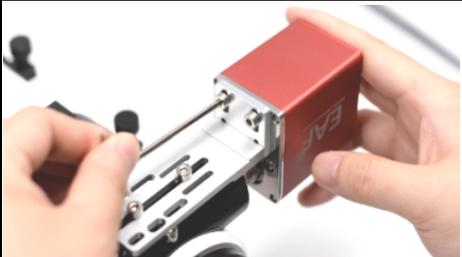
4 Secure the EAF body to the bracket and the bracket to the matching mounting holes in the focuser assembly using the supplied screws
