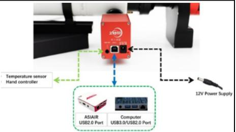
Connect the EAF to a 12V power supply # Control it through USB port or Hand controller.
