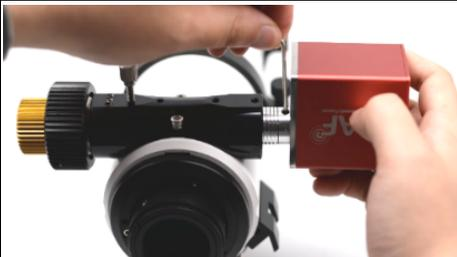
3 Attach the focuser body to the flexible coupler and tighten the lock screw using the supplied wrench
