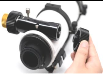
1 Remove the coarse adjustment knob of the telescope focuser using a suitable sized wrench
