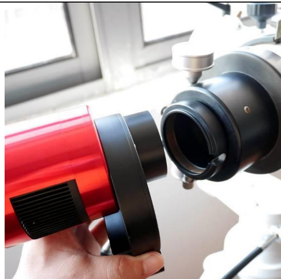
T2 extender can be used for attaching the telescope with 2" interface.
