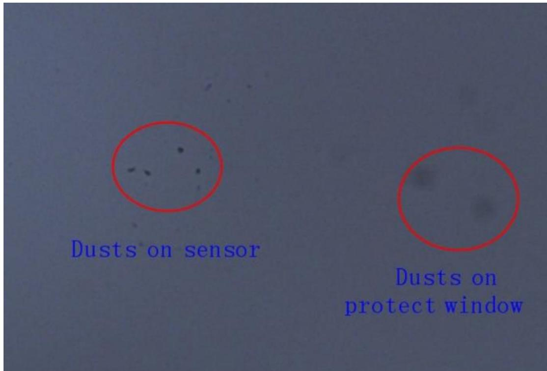
The big dim spot on the image (at right) are the shadows of dust on the protective window.
